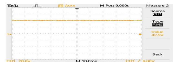
Figure shows a boost operation of constant output dc voltage of 42.5V for a 12V dc input.
